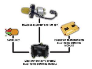
Each yellow or gray security key has a unique identification number. When a key is inserted into the ignition switch, the Cat Machine Security System electronic control module checks that key against the preapproved list. If the key is an unauthorized security key, or a standard black key, the machine will not start.
